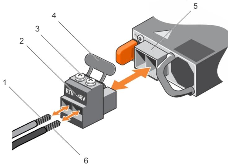
Figure 41. Assembling the DC input power wires
