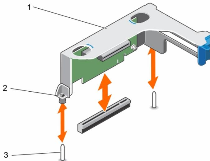
**Figure 26. Removing and installing the expansion card riser**
