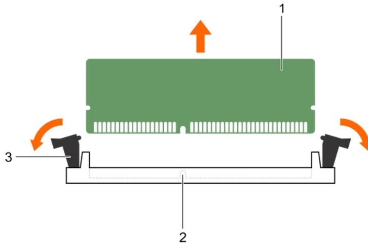
**Figure 15. Removing and installing a memory module**
