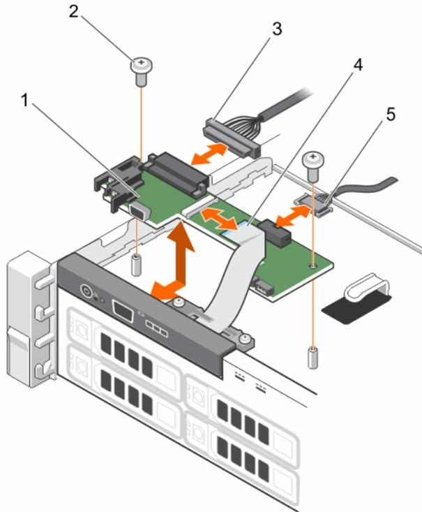
**Figure 47. Removing and installing the control-panel board**
