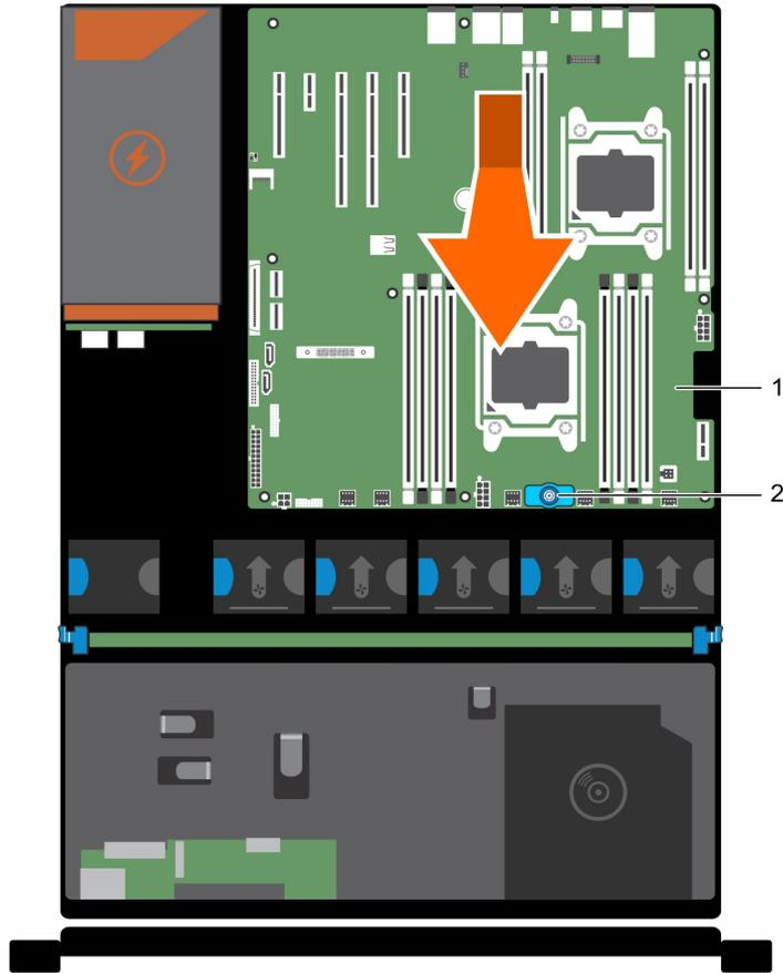
Figure 50. Removing and installing the system board
