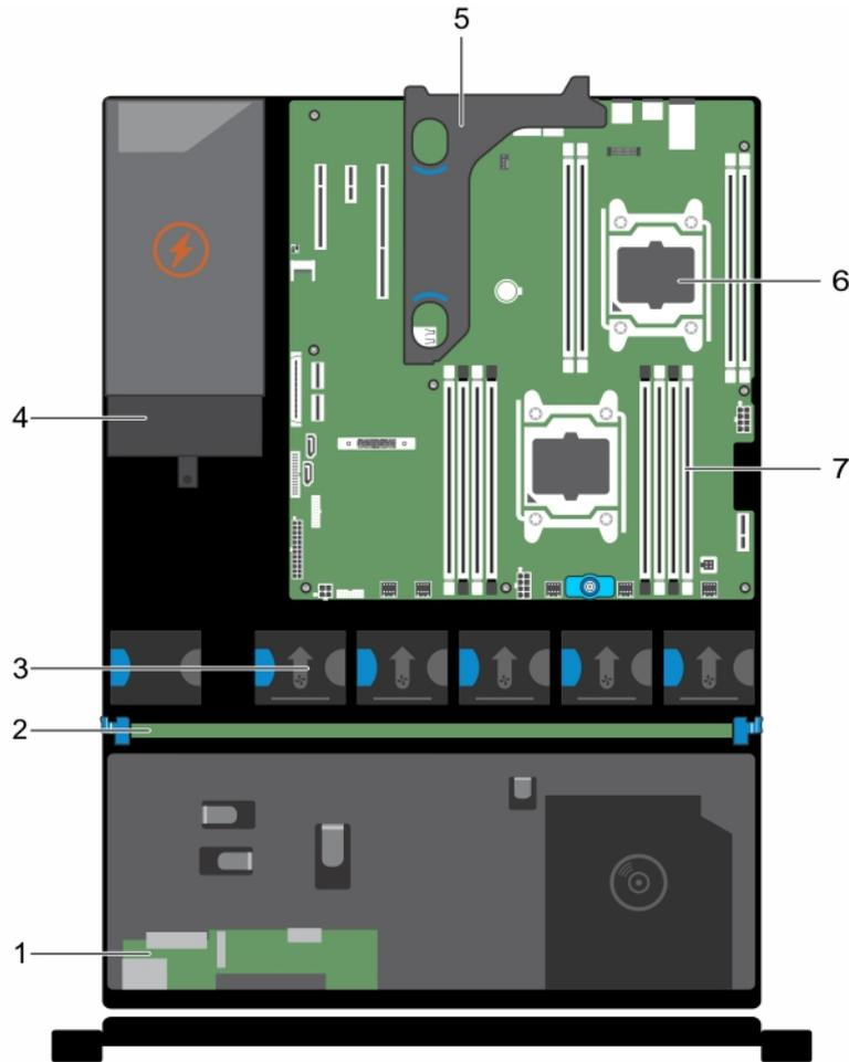
Figure 12. Inside the System—Non-Redundant Power Supply Unit Chassis
