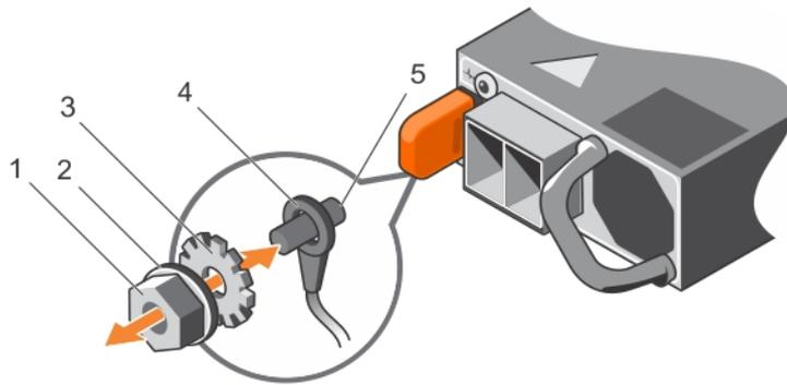
**Figure 40. Assembling and connecting the safety ground wire**
