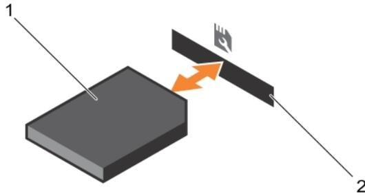
**Figure 30. Removing and installing the SD vFlash media card**
