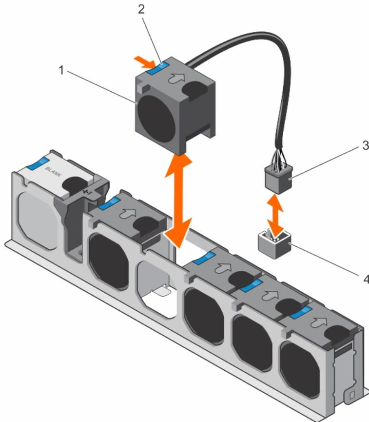
**Figure 24. Removing and installing a cooling fan**
