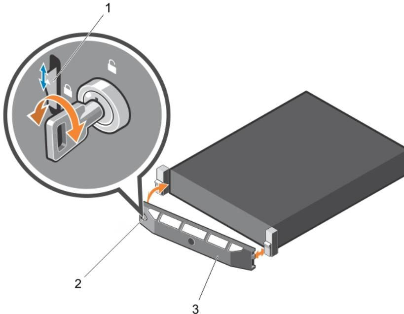
Figure 9. Removing and installing the front bezel
