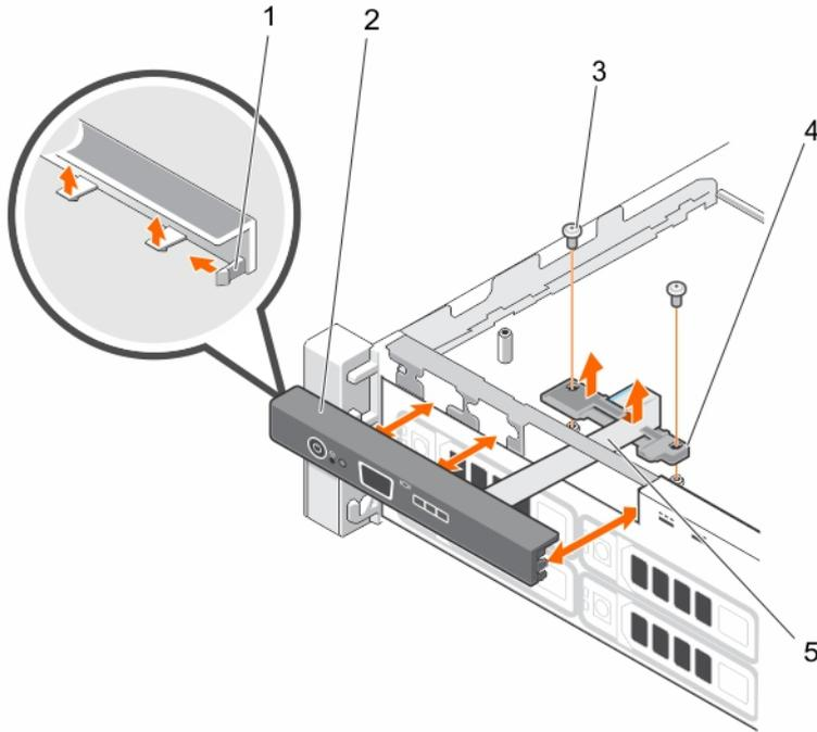
**Figure 48. Removing and installing the control panel**
