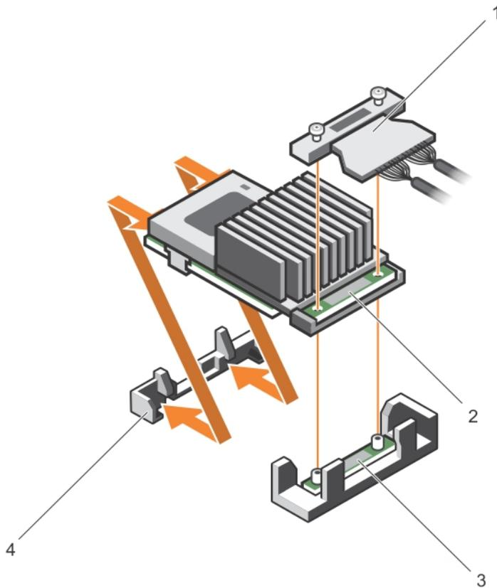
**Figure 32. Removing and installing the integrated storage controller card**
