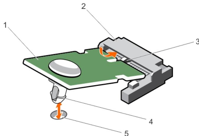
**Figure 51. Installing the TPM**
