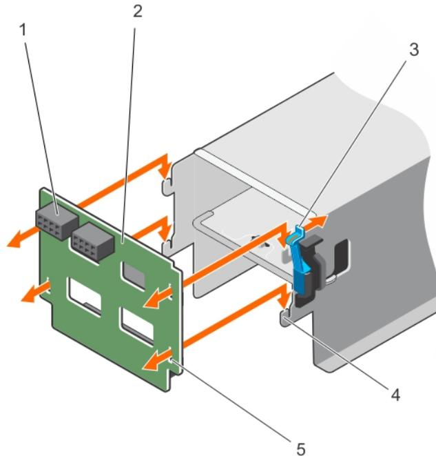
**Figure 43. Removing and installing the power interposer board**
