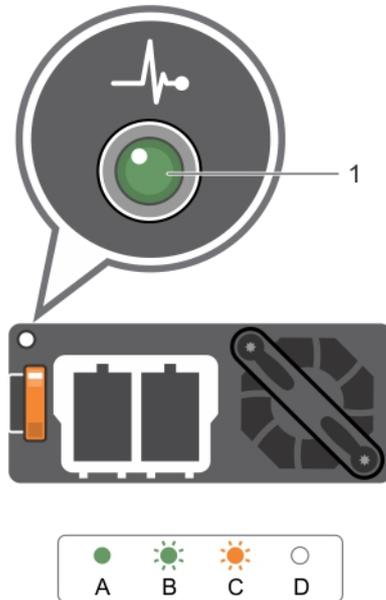
Figure 7. DC power supply unit status indicator
