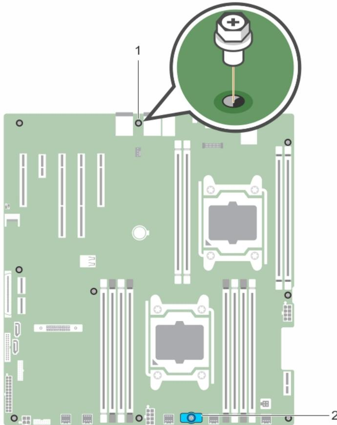
**Figure 49. Screw location on the system board**
