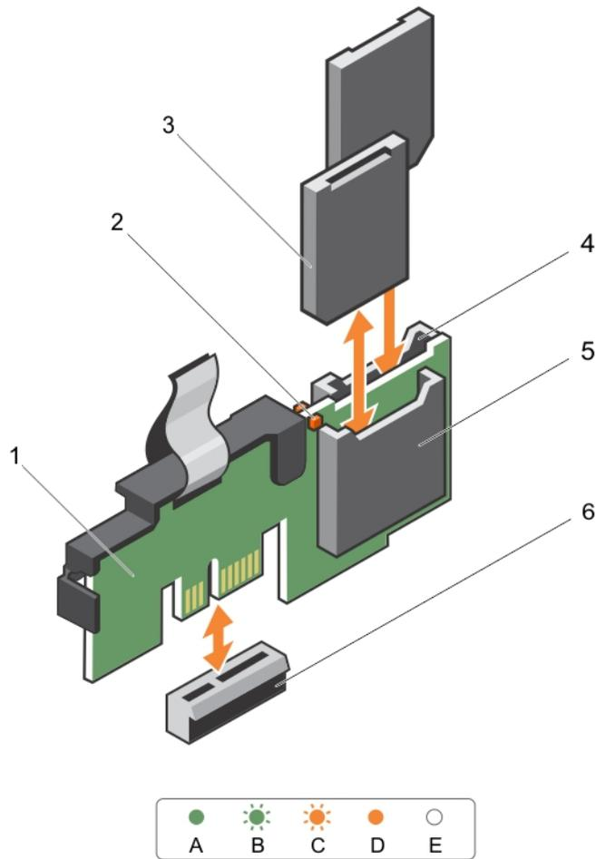
**Figure 31. Removing and installing the Internal Dual SD Module (IDSDM)**
