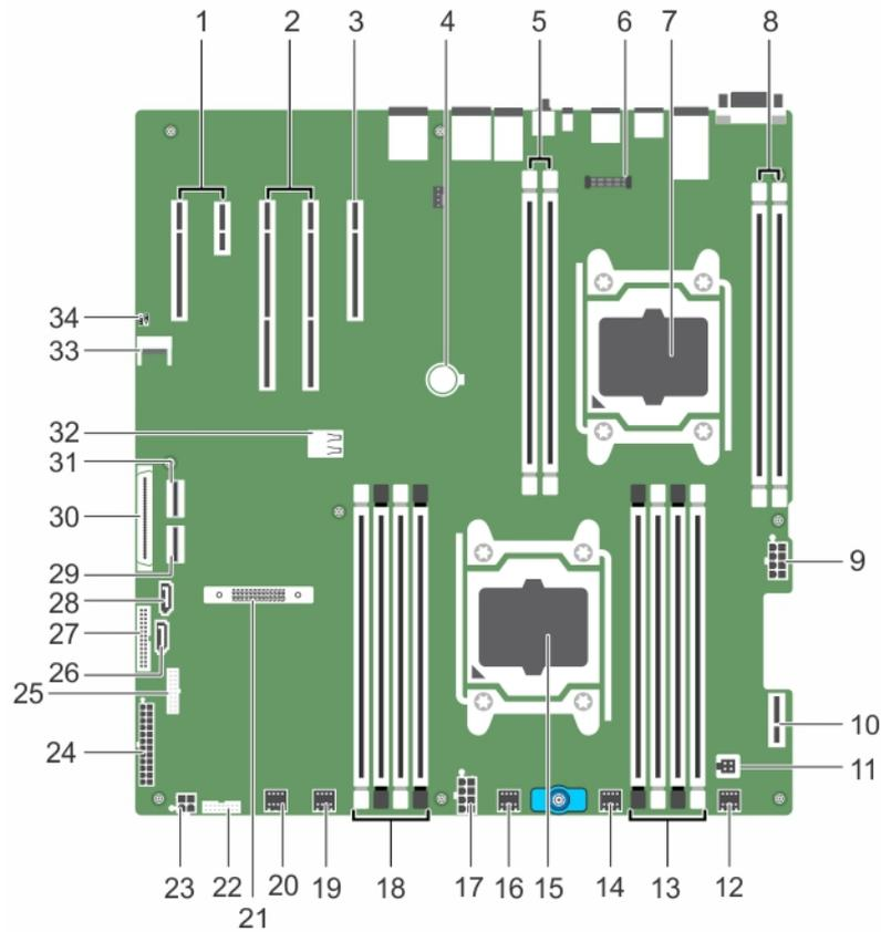
Figure 52. System board connectors and jumpers
