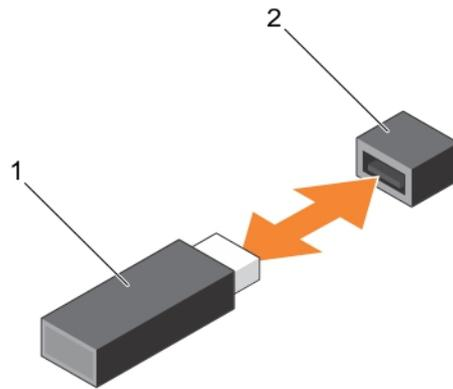
**Figure 25. Replacing the internal USB key**
