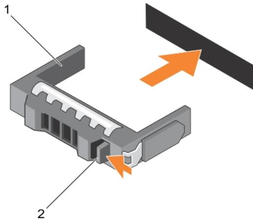
**Figure 18. Removing and installing a 3.5 inch hard-drive blank**
