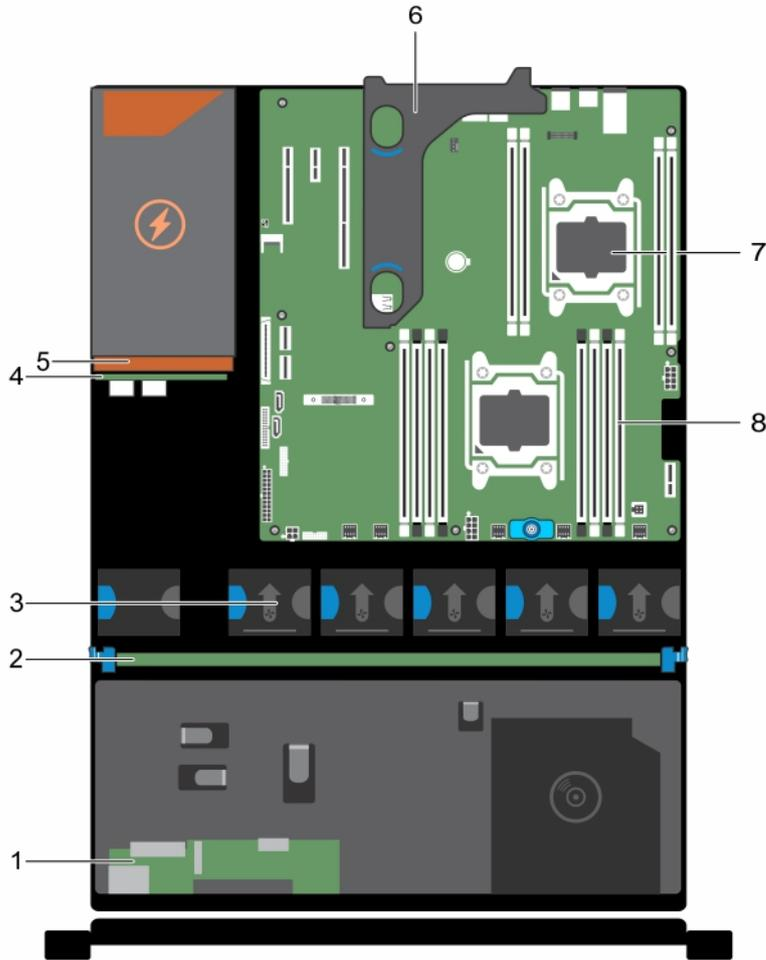
**Figure 11. Inside the System—Redundant Power Supply Unit Chassis**
