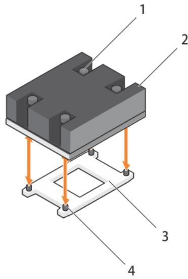
**Figure 33. Removing and installing a processor heat sink**
