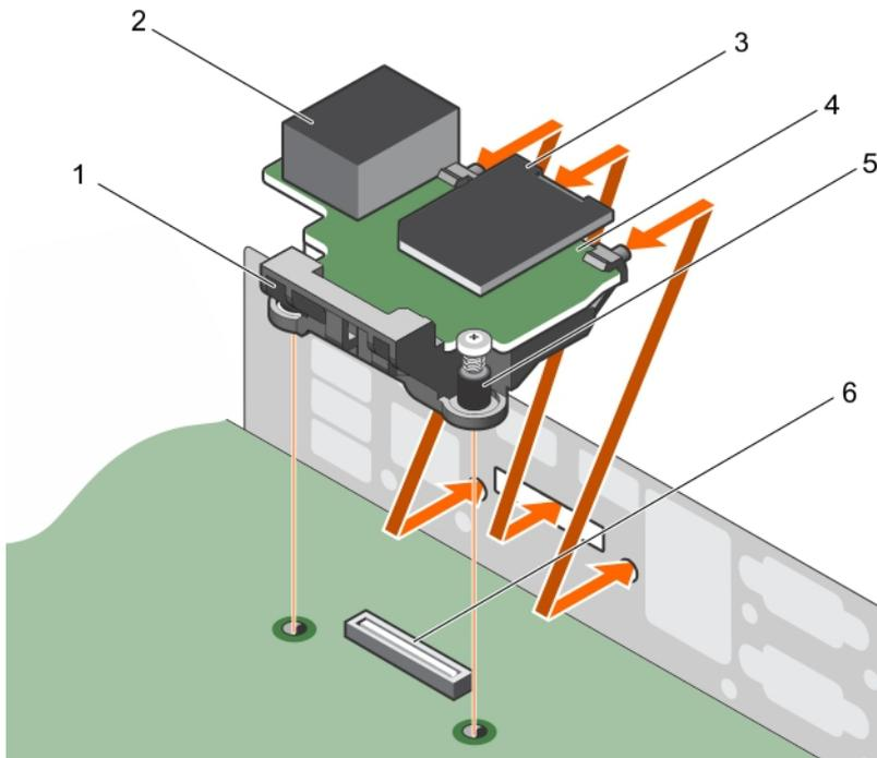
**Figure 29. Removing and installing the iDRAC ports card**
