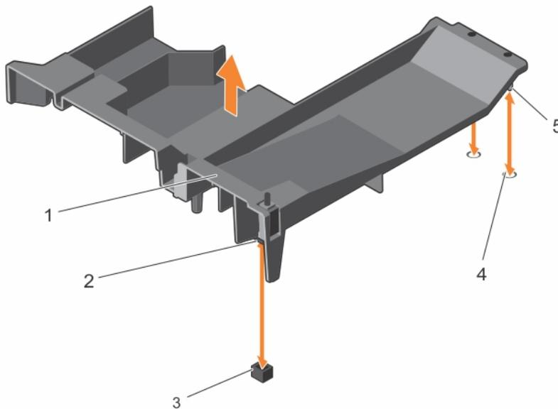
**Figure 13. Removing and installing the cooling shroud**
