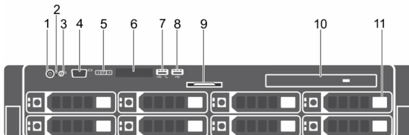
Figure 1. Front-panel features and indicators
