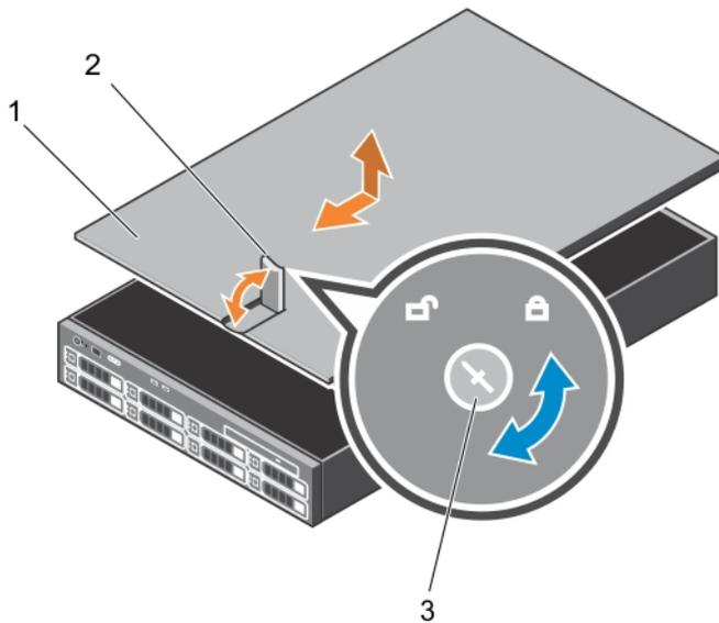
Figure 10. Opening and closing the system
