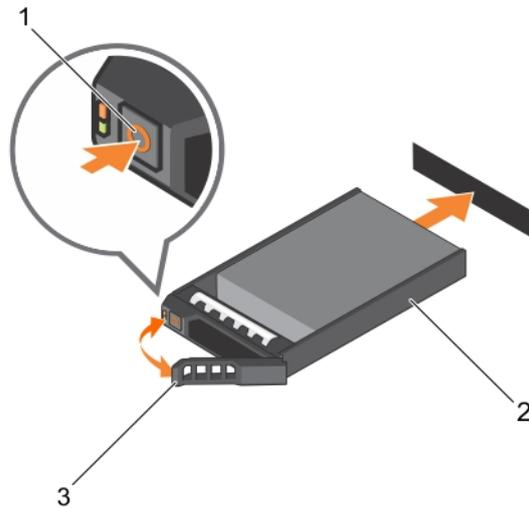
**Figure 17. Removing and installing a hot-swap hard drive**
